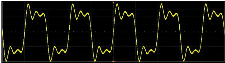
Figure 2-6: Square pulses distorted at high frequencies
