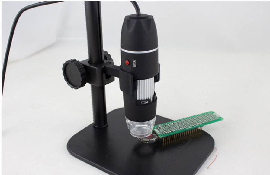
Figure A-12: A low-cost USB microscope
