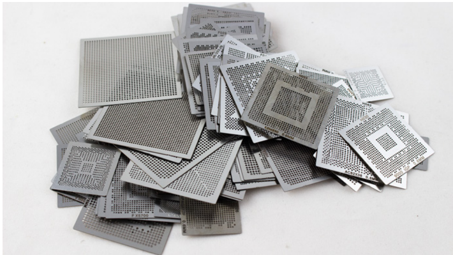
Figure A-7: Example of a cheap set of stencils for BGA reballing
