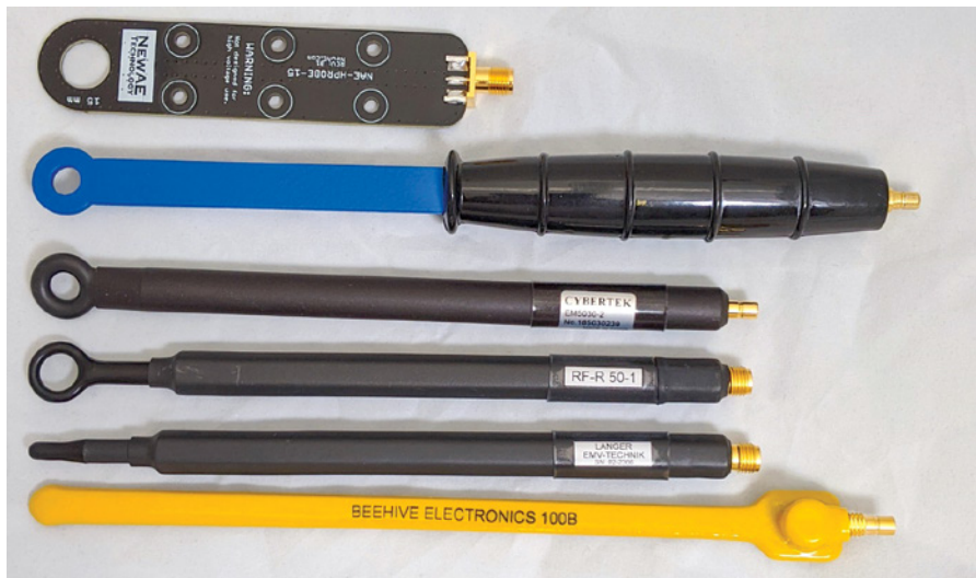
Figure A-26: H-Field probes from various manufacturers
