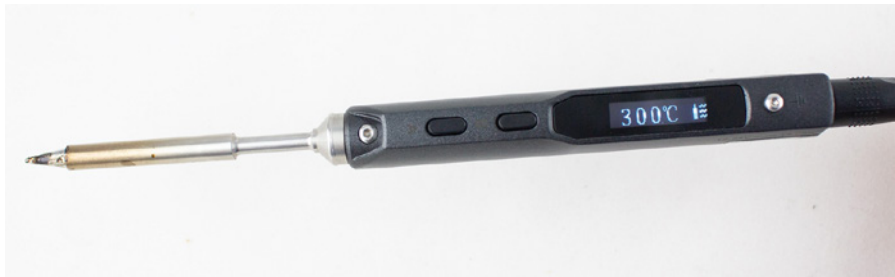
Figure A-4: The TS100 is a low-cost iron that performs well relative to higher-priced irons.
