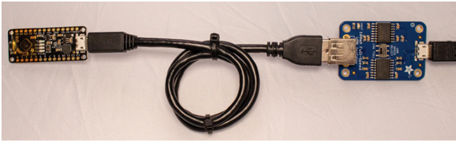
Figure 6-3: An isolator from Adafruit (PCB on the right) and our target (PCB on the left)
