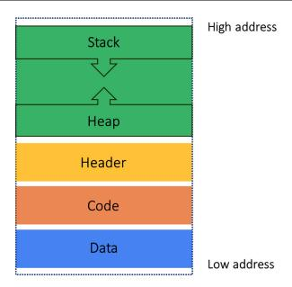
Figure 2.3 – Illustration of a process' virtual memory
