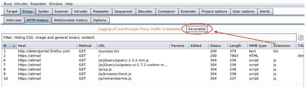
Figure 27: Re-enabling the outof-scope traffic capture
