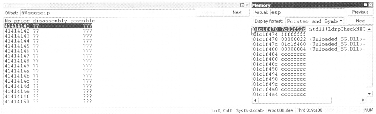
Figure 21: Stack frame layout in LdrpCheckNxCompatibility epilogue (after RETN 0x4)
