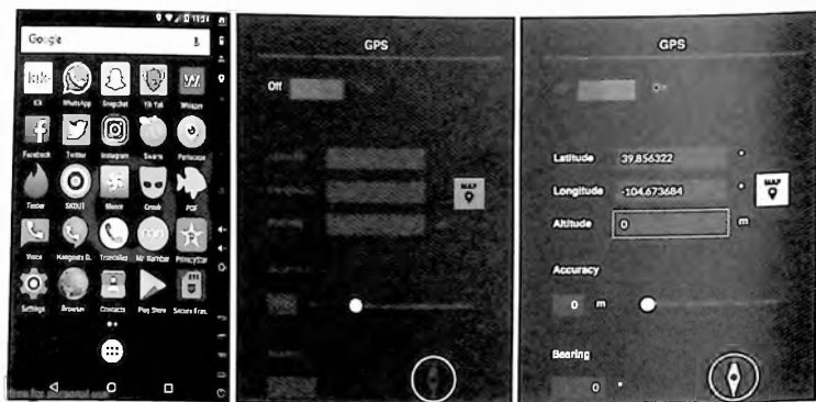
Figure 7.04: A custom Android emulator home screen with several apps installed into groups (left), disabled Genymotion GPS menu (middle) and spoofed GPS (right).
