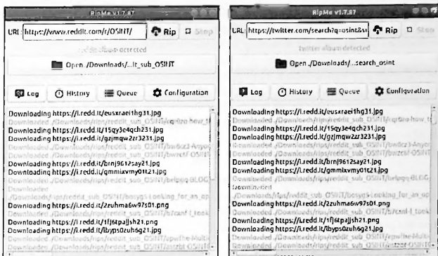
Figure 4.09: The RipMe application extracting bulk images from Reddit and Twitter.
