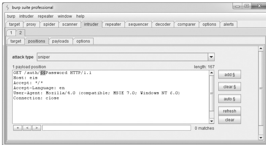
Figure 4-7: Burp Intruder being used to perform a customized brute-force attack on part of a filename
