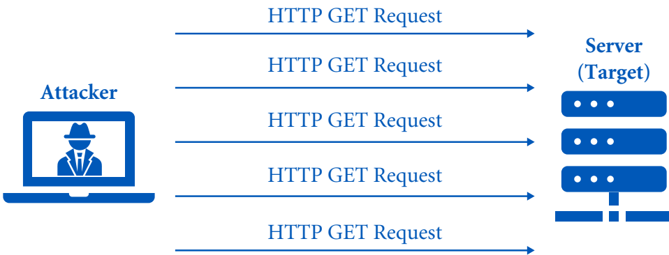
FIGURE 6.16 A Slowloris attack with unfinished simultaneous HTTP request.
