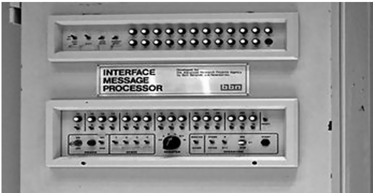
FIGURE 5.2 The first routers, known as Interface Message Processors or IMPs. Courtesy of DARPA.
