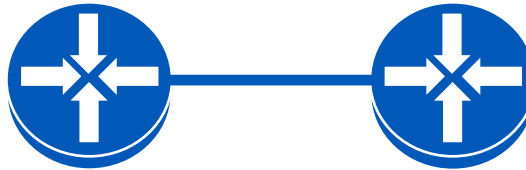
FIGURE 5.32 A point-to-point connection between two routers.
