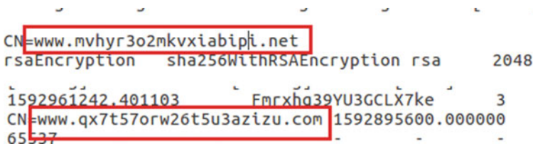
Fig. 30 Bro/Zeek deep packet analyzer—shows us the user was browsing tor network
