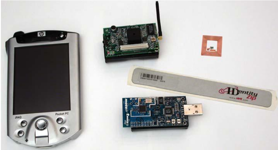
FIGURE 5.2 Examples of embedded devices: PDA, sensors, and RFID tags.
