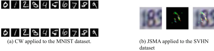
Fig. 2 (a) Top row : MNIST adversarial examples targeted for 0. Bottom row : MNIST adversarial examples targeted for 1. (b) JSMA adversarial features visualized
