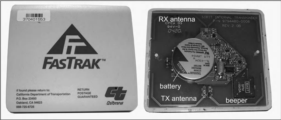
Figure 2.20 Commercial semi-passive tag: external view (left) and internal circuitry (right).
