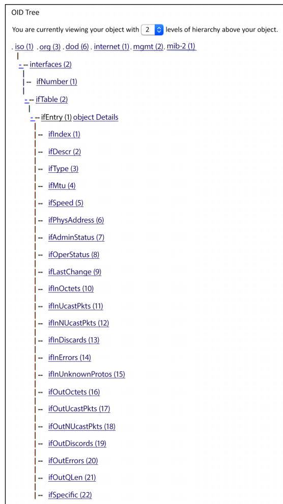
Figure 7.3: SNMP ifEntry OID tree
