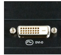
Figure 1.8 HDMI and DVI are common types of video input ports found on modern TVs and monitors. It's easiest to connect a Raspberry Pi to a TV or monitor with an HDMI port. HDMI provides a high-definition picture and doesn't require any adapters or converters—only an HDMI cable, which is included in many Pi kits. The DVI port requires a special adapter to connect with a Pi.
