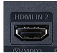
Figure 1.8 HDMI and DVI are common types of video input ports found on modern TVs and monitors. It's easiest to connect a Raspberry Pi to a TV or monitor with an HDMI port. HDMI provides a high-definition picture and doesn't require any adapters or converters—only an HDMI cable, which is included in many Pi kits. The DVI port requires a special adapter to connect with a Pi.
