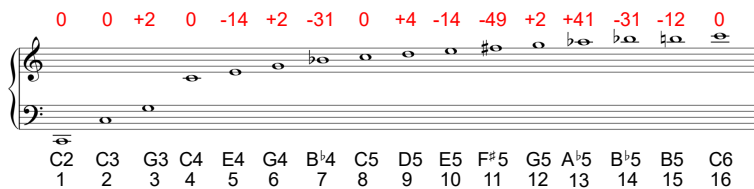
Fig. 1.20 Illustration of the harmonic series in music notation. Starting with the note C2, for each of the first 16 harmonics the closest musical note is shown. On top, the difference (in cents) between a harmonic’s frequency and the center frequency of the closest note is shown.
