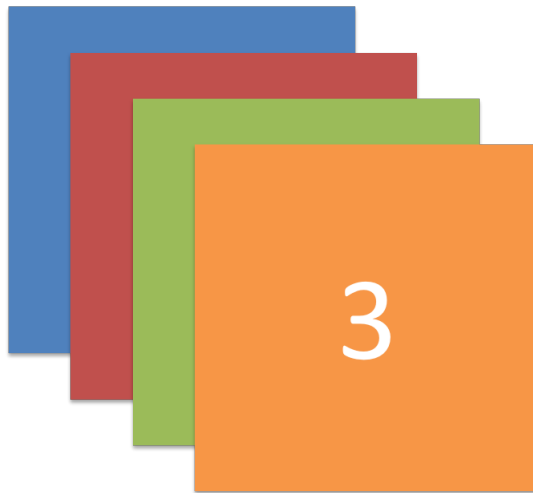
Figure 31. QStackedLayout — in use only the uppermost widget is visible, which is by default the first widget added to the layout.
