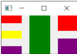
Figure 27. Nested QHBoxLayout and QVBoxLayout layouts with spacing and margins around the widgets.
