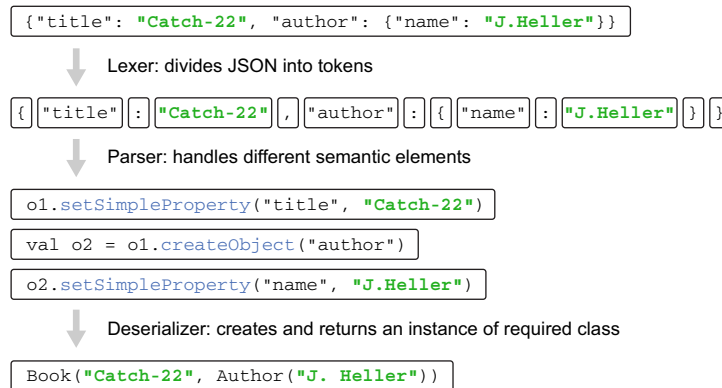
Figure 10.7 JSON parsing: lexer, parser, and deserializer
