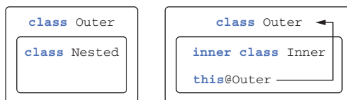
Figure 4.1 Nested classes don't reference their outer class, whereas inner classes do.
