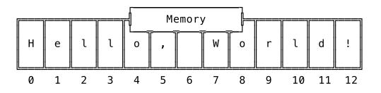
The letter "H" has the memory address 0, "e" has 1, the first "l" has 2, "W" has 7 and so on. We could access every single letter of the string Hello, World! by using the memory addresses 0 to 12. "Hey CPU, fetch the word at memory address 4" would result in the CPU fetching the letter "o". Straightforward, right? I know what you're thinking right now and, yes, if we take such a number – a memory address – and save it to another place in memory, we create a pointer.
