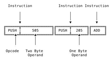
This helps to illustrate the general idea, but bytecode is a binary format and not nearly as readable. Meaning that you can't read it like a text file. The mnemonics, like PUSH, don't show up in the actual bytecode. They are replaced by the opcodes they refer to, and those are just numbers – bytes. Which numbers exactly is up to the person defining the bytecode. The PUSH mnemonic might stand for the number 0 and POP might refer to the number 23.
