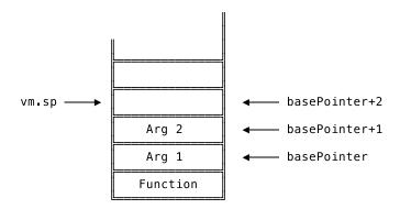
That would work. With this, if we'd compute basePointer *plus* local binding index of the argument, we'd get the correct slot. And on top of that (pun intended!) the vm.sp would still point to the next empty slot on the stack. Perfect!
