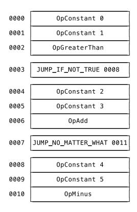
The operand of  $JUMP_IF_NOT_TRUE$  is now 0008. That's the index of the OpConstant 4 instruction to which the VM should jump in case the condition is not true. The operand of  $JUMP_NO_MATTER_WHAT$  is 0011, which is the index of the instruction following the whole conditional.
