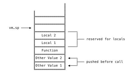
We already have the necessary parts to pull this off: the value of the stack pointer before executing the function, giving us the lower boundary of the hole, and an index that increases with every local. We can use both to calculate a stack slot index for each local binding by adding them together. Every index calculated this way serves as an offset into the hole and points to the slot where we'll store the local binding.
