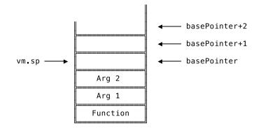
I bet you can see the problem. We set basePointer to the current value of vm.sp *after* we pushed the arguments on the stack. That leads to basePointer *plus* the index of the local binding pointing to empty stack slots. And the result of that is that the VM gets nils instead of the arguments it wants.
