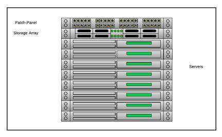
The components of a rack (server blades, network switches, and so on) are often classified in terms of their sizes or Rack Unit. This is a unit of measure used to describe the height of a device mounted in a 19-inch rack or a 23-inch rack and is approximately 44.45 mm (1.75 inches) high. Device form factors are often in terms of multiples of rack units (1U, 2U, and so on).
