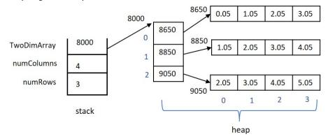
Figure 3.4 – Memory model for Chp3-Ex4.cpp
