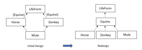
Figure 9.2 – Diamond-shaped multiple inheritance redesigned without MI
