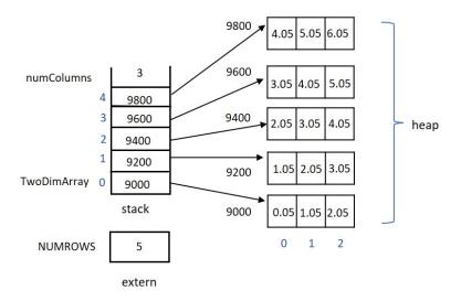
Figure 3.3 – Memory model for Chp3-Ex3.cpp
