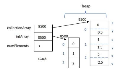
Figure 3.2 – Memory model for Chp3-Ex2.cpp
