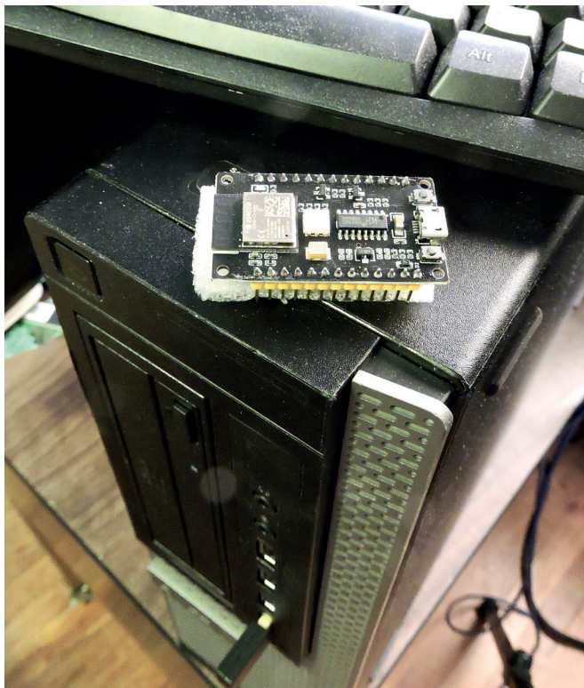
Figure 3.1: Size contrast of the ESP32-C3 dev board with a typical Windows-10 tower.
