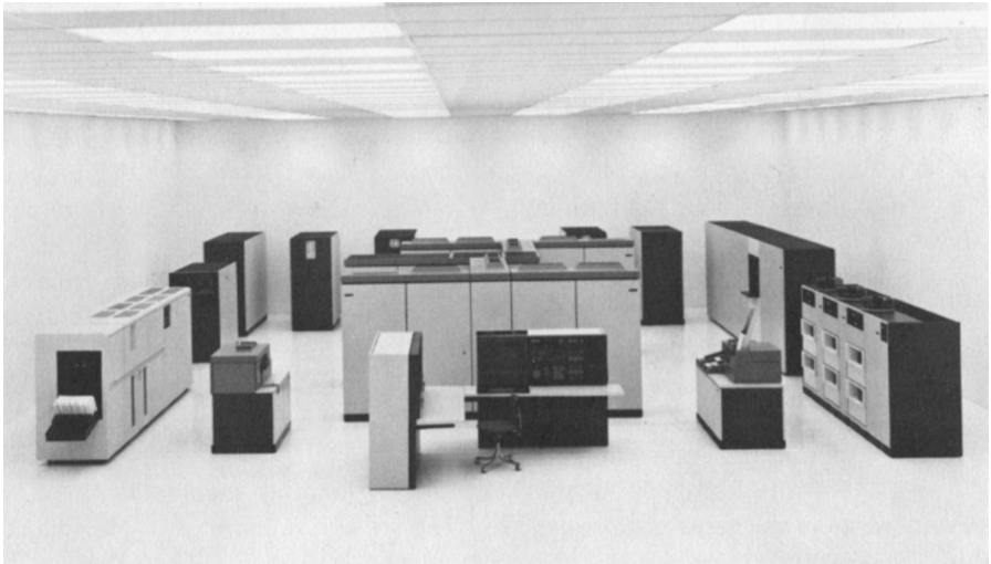
FIGURE 10.15 An IBM Model 168. One of the most powerful computers available from IBM is shown here with a complete set of peripheral devices. (Photo courtesy of IBM Corporation.)
