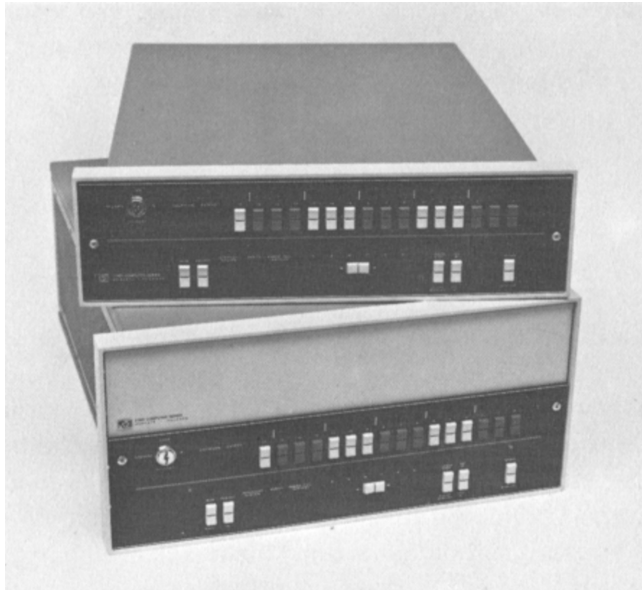
FIGURE 10.6 Two of the HP 21MX series of computers from Hewlett-Packard. These small minicomputers are often used in dedicated applications. (Photo courtesy of Hewlett-Packard Company.)
