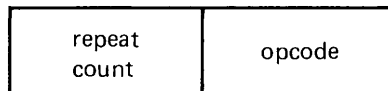
FIGURE 10.25 Instruction format in character mode. Each instruction has a 6-bit repeat count and a 6-bit opcode. All operations are between two memory areas, the source character string and the destination character string.
