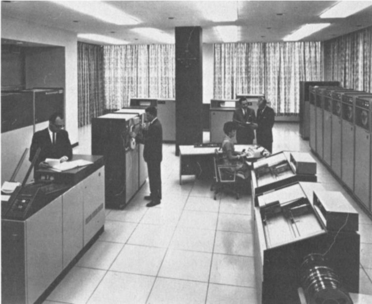
FIGURE 10.21 A Burroughs B5500 computer system. The B5500 was a very successful computer system based on a stack architecture. (Photo courtesy of Burroughs Corporation.)
