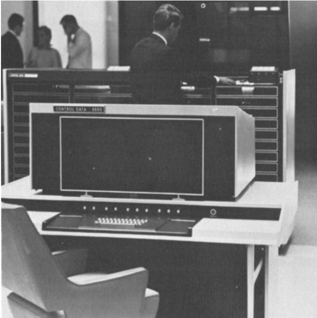
FIGURE 10.26 A CDC 6600. The 6600 is composed of 11 separate computers: one central processor and 10 peripheral processors. One peripheral processor is commonly used to drive the operator's console, shown in the foreground. (Photo courtesy of Control Data Corporation.)
