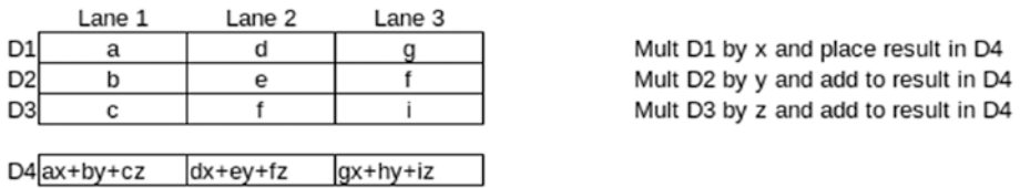
Figure 12-4. Showing how the calculations flow through the lanes
