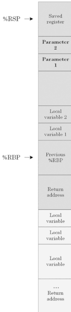
Figure 11-1. Stack memory layout for the function with two arguments and two local variables
