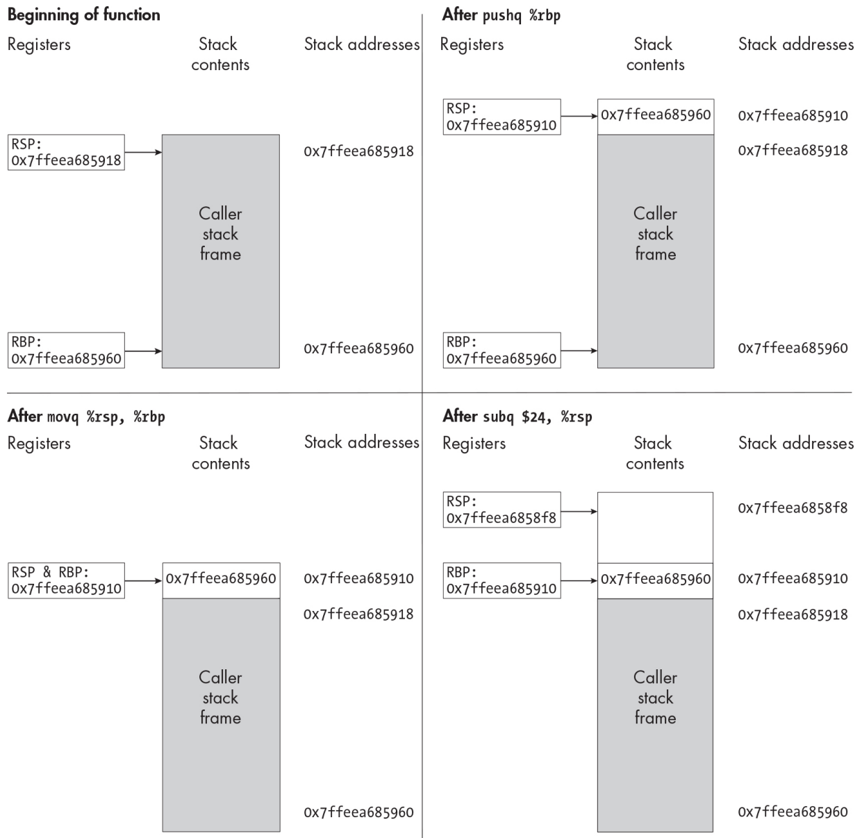
Figure 2-2: The state of the stack at each point in the function prologue Description
