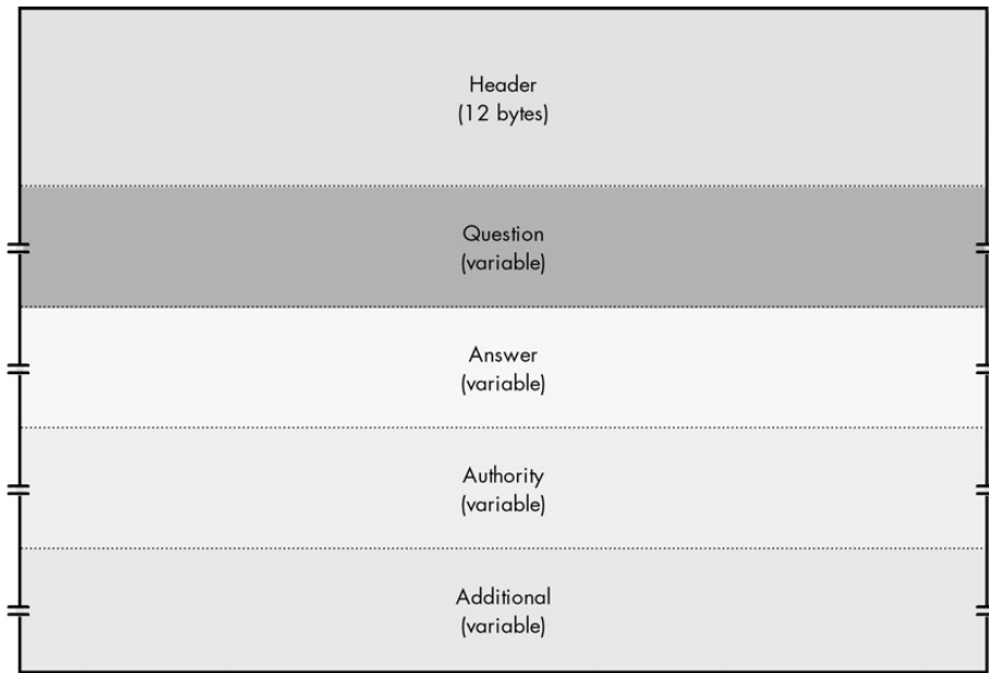
Figure 57-1: DNS general message format
