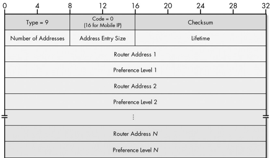
Figure 33-3: ICMPv4 Router Advertisement Message format
