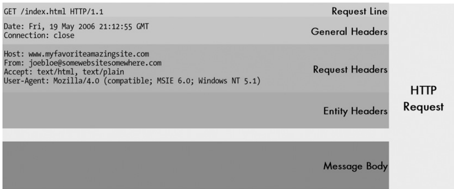
Figure 81-1: HTTP Request message format This diagram shows the structural elements of an HTTP Request message and an example of the sorts of headers a Request message might contain. Like most HTTP requests, this one carries no entity, so there are no entity headers and the message body is empty. See Figure 81-2 for the HTTP Response message format.
