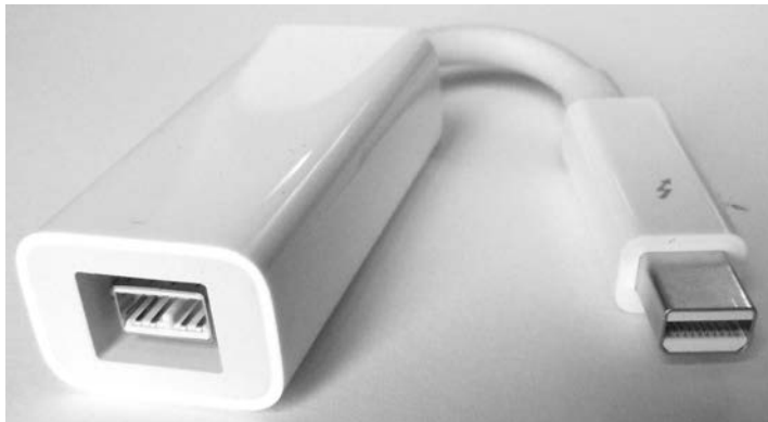
Figure 5-4: Thunderbolt to Firewire adapter
