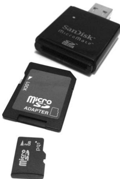
Figure 6-1: Removable memory card adapters
