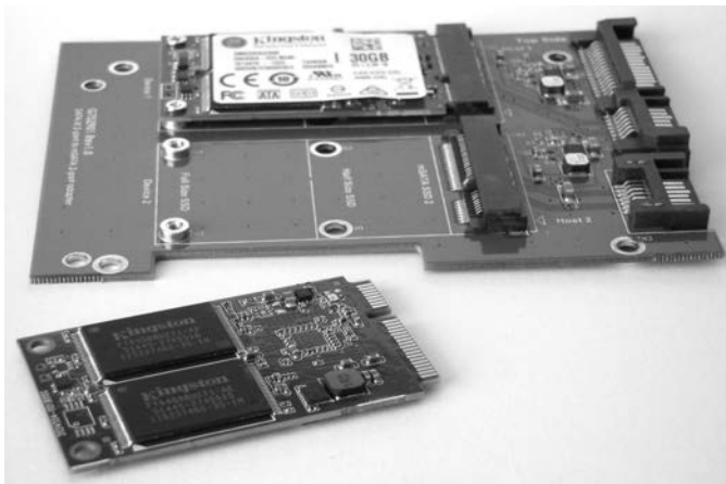
Figure 1-9: mSATA disk interface
