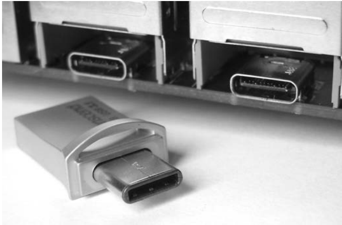
Figure 1-20: USB Type C interface
