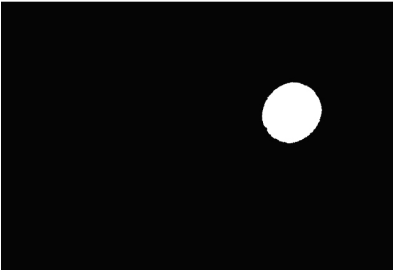
Figure 15-6: Screen capture of one of the original video frames converted to pure black and white
