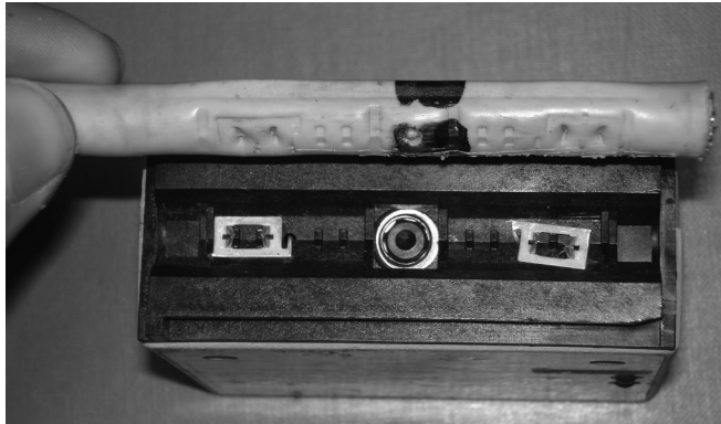
Figure 6-3: Example of a vampire tap (image modified from the original covered by the Attribution-ShareAlike 2.5 Generic [CC BY-SA 2.5] license, https://creativecommons.org/licenses/by-sa/2.5/ )
