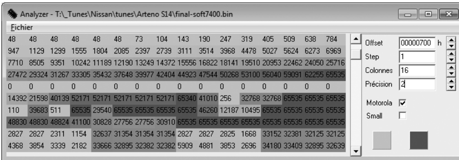
Figure 6-4: VQ table in analyze.exe: values from 48 to 65535 in first four rows of 16x16-bit values
