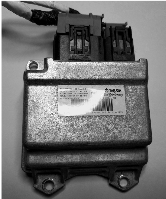
Figure 4-1: A typical event data recorder
