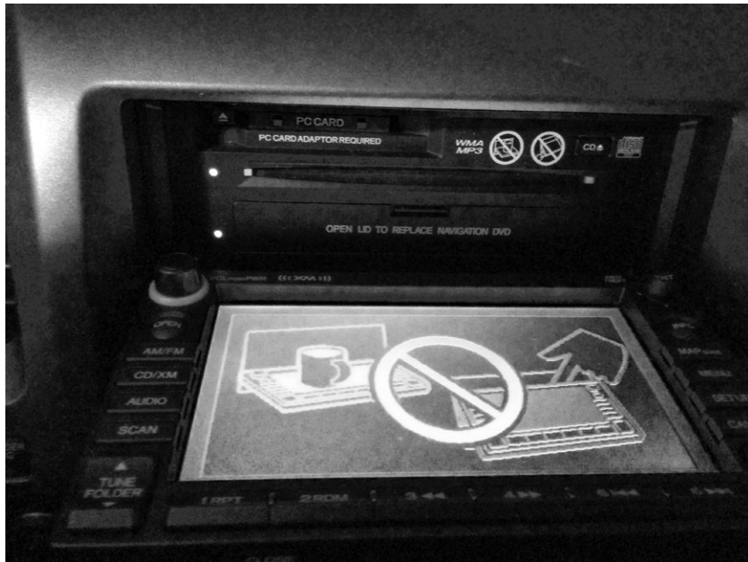
Figure 9-1: NavTeq infotainment unit in an open state
