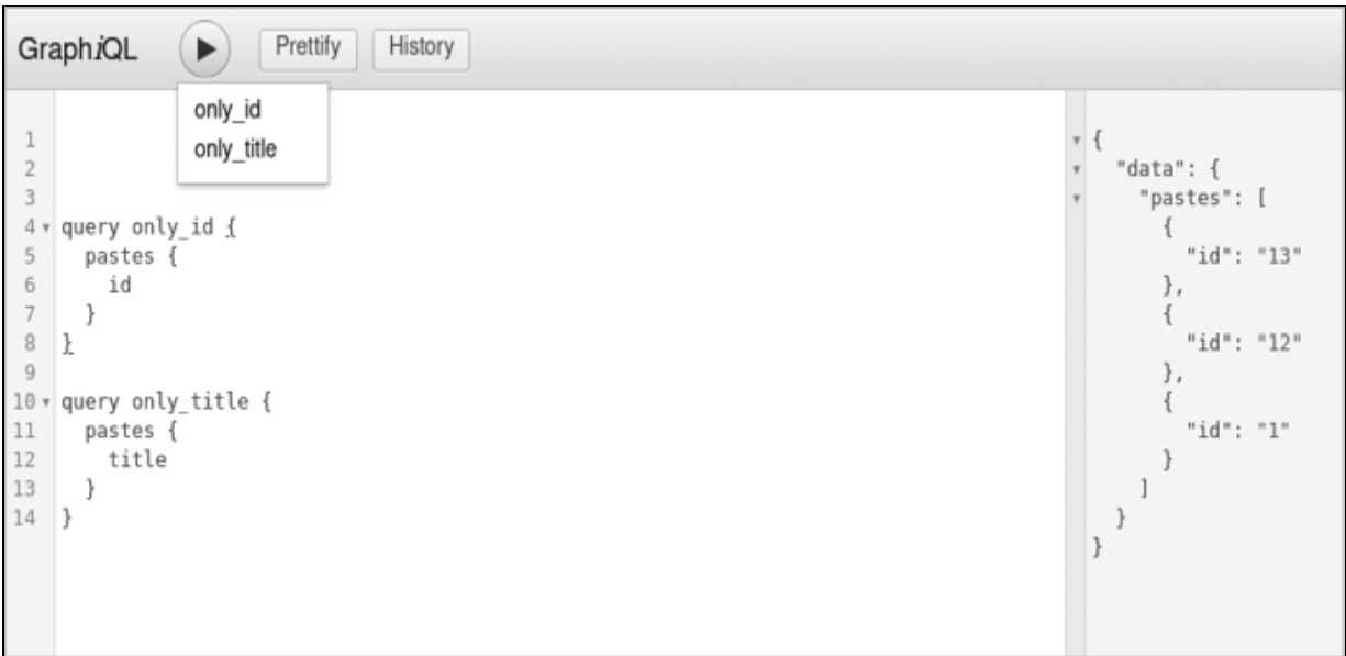
Figure 8-2: Executing a selected query based on its operation name in GraphiQL Explorer
