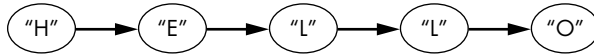
Figure 4-3: A linked list data structure storing HELLO . Linked lists can be considered a kind of tree data structure.
