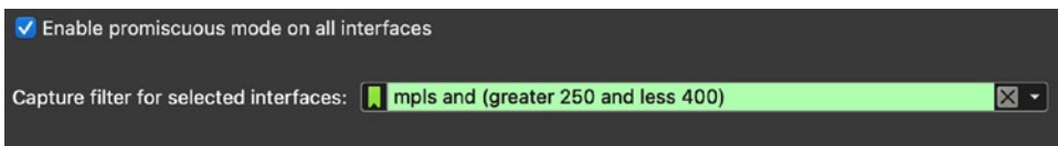
Figure 2-18. Capture filter for MPLS packets 250–400 bytes
