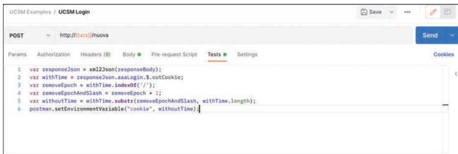
Figure 16-33 Creating the Test to Gather the UCSM API Cookie from the Response Payload
