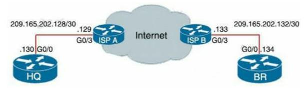
BR(config)#interface tunnel1 BR(config-if)#keepalive 5 3 HQ(config)#interface tunnel1 HQ(config-if)#keepalive 5 3
