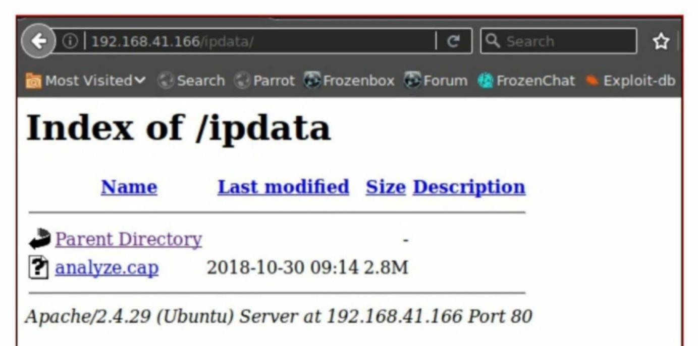
This url has a file named analyze.cap. That's strange. A CAP file is a packet capture file. By packets we mean the traffic that goes from one device to another in a computer network. This file is generally created by a packet sniffer and can only be opened with a sniffer. Let's analyze this file using Wireshark. We download the file analyze.cap.
