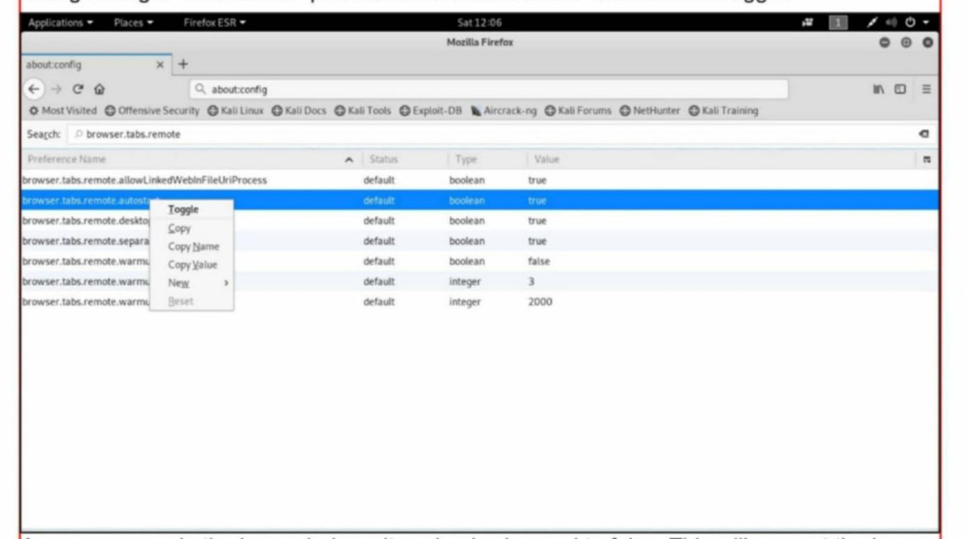
As you can see in the image below, its value is changed to false. This will prevent the brows -er from automatically reloading all the tabs which will slow down the firefox browser. This wil -I prevent the browser from automatically reloading all the tabs which will slow down the firefox browser.
