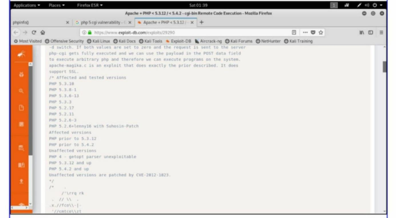
After doing a bit of research, it is revealed that PHP upto versions 5.3.12 and 5.4.2 when run as CGi is vulnerable to argument injection. Argument injection vulnerability is exploited by giv -ing a malformed argument. I searched for any exploits written for exploiting this particular vulnerability.
