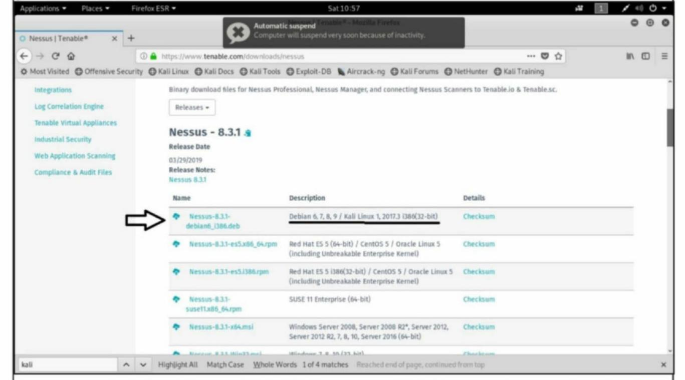
Since we are installing this on a i386 (32bit) version of Kali Linux, we here are downloading the i386 version of Nessus. If you have a amd64 (64bit) version of Kali Linux, scroll down on the Downloads webpage of Nessus to find that version of Nessus and download it. Otherwise we can also install the i386 version of Nessus in the amd64 version of Kali Linux.
