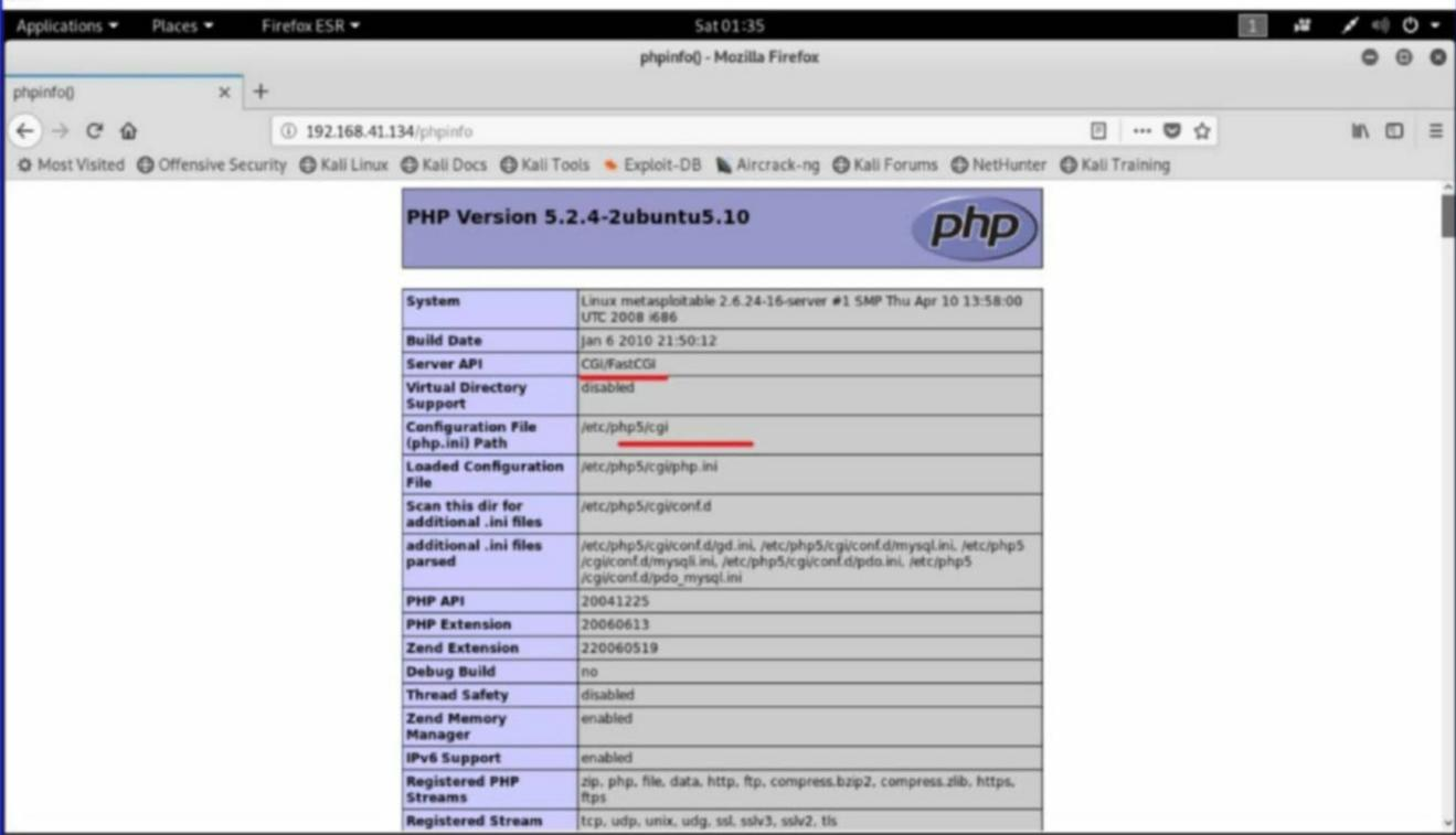
On observing the "phpinfo" page, we can see that PHP 5 is running on our target with CGI. CGI stands for Common Gateway Interface. It is mostly used for running web applications.
