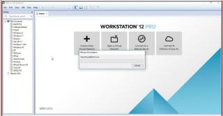
After the importing process is finished, a virtual machine is automatically created as shown b elow. No need to assign RAM or any other system specifications.
