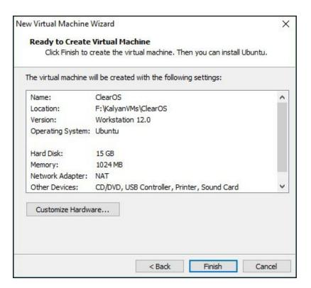
The virtual machine is created with the name you gave it. Before powering on the virtual machine, we need to add another network adapter to the virtual machine. Any gateway needs two network adapters. For reasons that will be explained later, I am adding two host only network adapters. Go to the settings of the virtual machine as shown below and click on "add" but ton as shown below.
