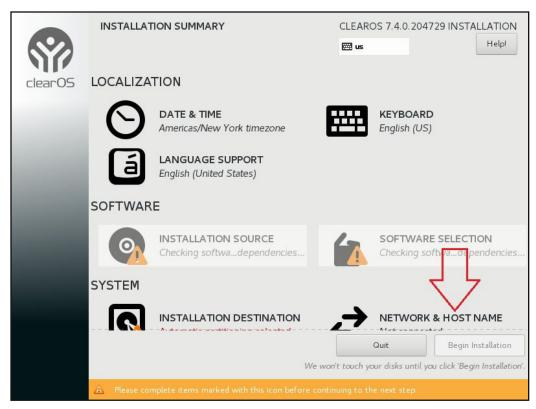
The "Network and Hostname" window will open. By default, both the adapters will be turned OFF. We need turn it ON by toggling the switch as shown in the image below.
