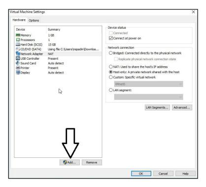
A new sub-window will open showing you all the types of hardware which can be added. Clic -k on the "network adapter" as we want to add a network adapter. Click on "Next".
