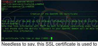
Needless to say, this SSL certificate is used to create an https connection for the web interface of OpenVAS scanner.
