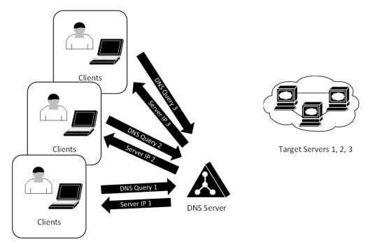
Figure 10.1 – Simple load balancing with Round Robin DNS
