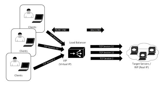
Figure 10.2 - Load balancing using a reverse proxy
