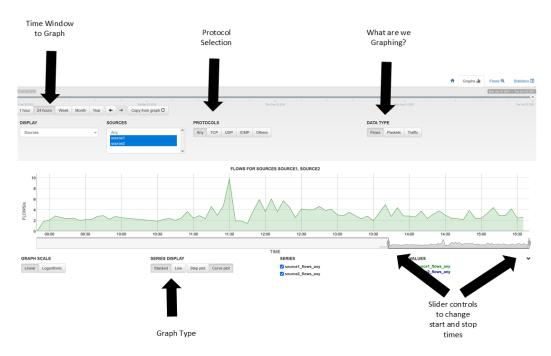
Figure 12.23 - Basic flow data in the graph display with display/filter controls in NFSen
