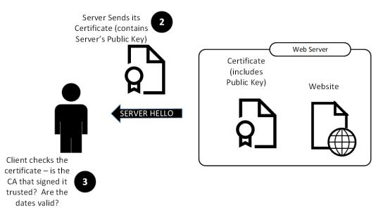
Figure 8.3 - TLS exchange: server hello is sent and certificate is validated by the client
