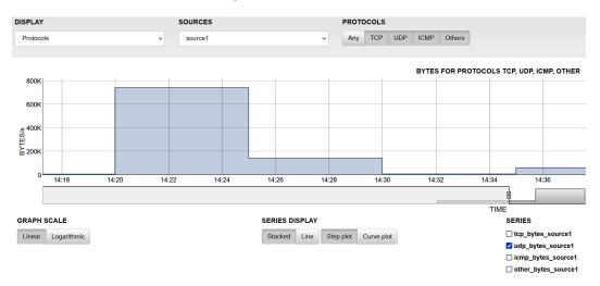
Figure 12.27 - Display adjustments in the protocol display, showing UDP only
