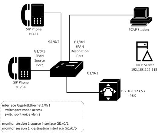
Figure 11.6 – Lab setup for packet captures
