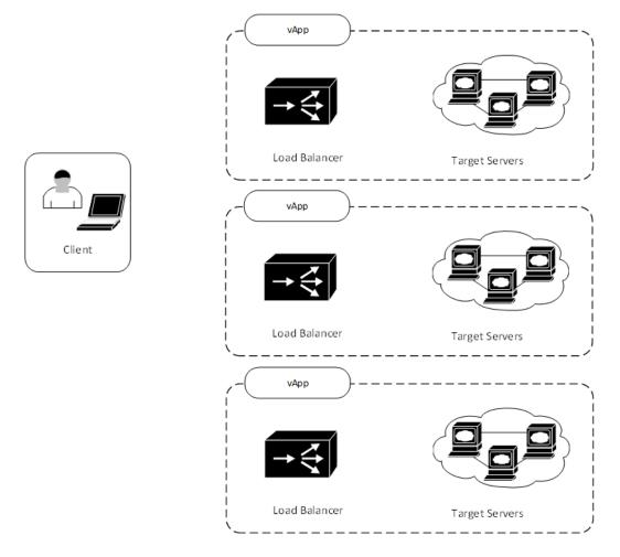
Figure 10.6 - Modern load balancing architecture
