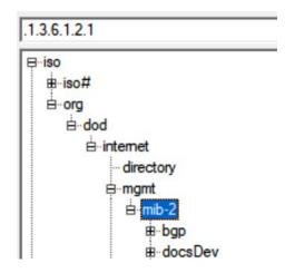
Figure 12.2 – SNMP OID tree, showing mib-2
