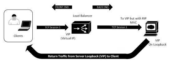
Figure 10.4 – DSR load balancing
