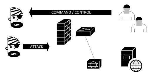
Figure 13.2 - IPS inside the firewall detecting C2 traffic. Also, some internet "noise" is filtered out
