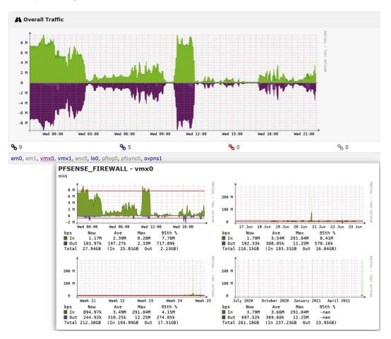
Figure 12.11 - Mousing over an interface for interface details in LibreNMS
