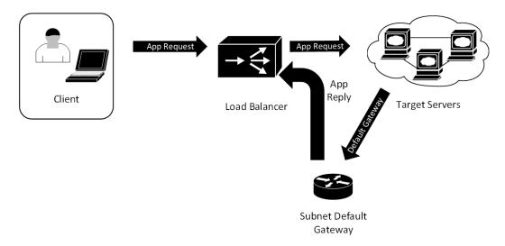
Figure 10.8 - Routing non-application traffic - policy routing on an upstream router
