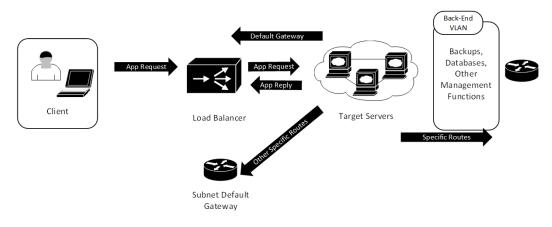
Figure 10.7 - Routing non-application traffic (high level)
