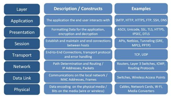
Figure 3.1 - The OSI model for network communication, with some descriptions and examples
