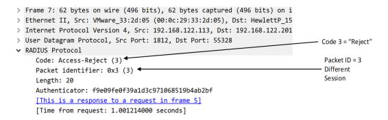
Figure 9.3 – Simple RADIUS response (Access-Reject)
