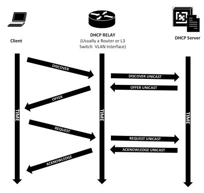
Figure 7.3 – DHCP relay or forwarder operation
