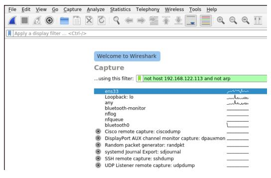
Figure 11.4 – Adding a capture filter to Wireshark
