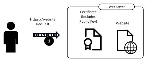
Figure 8.2 – TLS communication starts with a client hello
