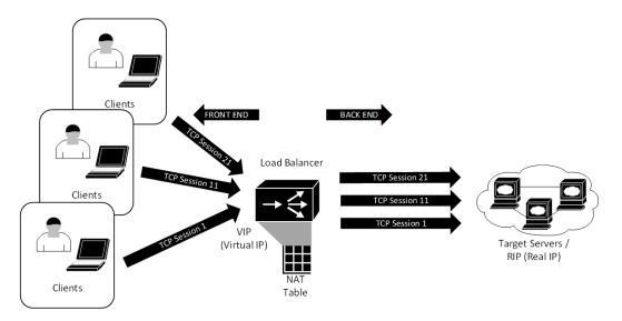
Figure 10.3 – Load balancing using inbound NAT
