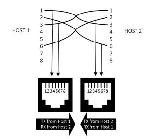
Figure 11.1 – Two tap ports, each in one direction
