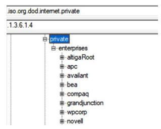
Figure 12.4 - SNMP OID tree, showing the Vendor OID section
