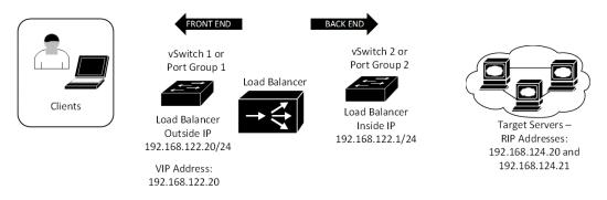
Figure 10.10 – Load balancer example build
