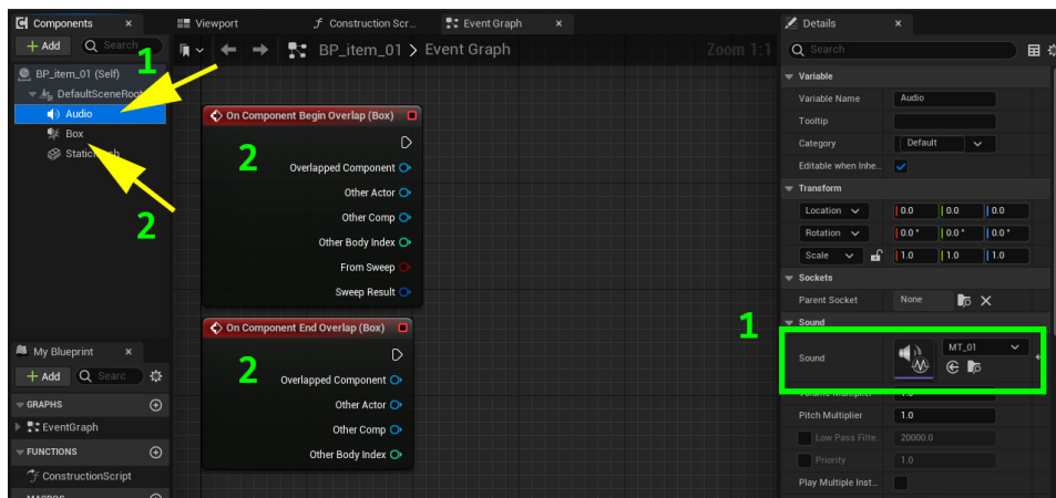
Figure 11.33: Select Audio component and assign “MS_01” MetaSound object for its Sound property (1), also bind collision events for box component(2).
