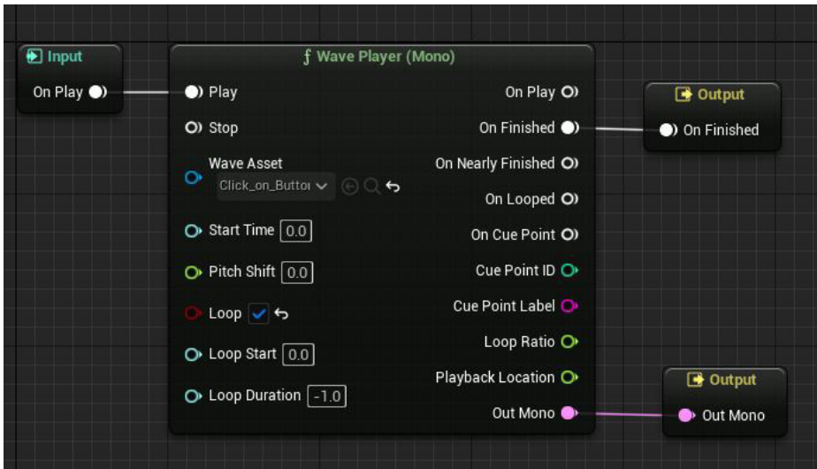
Figure 11.36: Check “Loop” check box in WavePlayer box to for looping the sound
