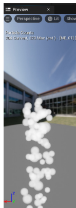
Figure 11.10: Falling effect on sprites by using Gravity Force module
