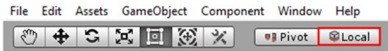
Figure 17-1. The Tool Handle Rotation, highlighted with a red box, is shown in the Local setting
