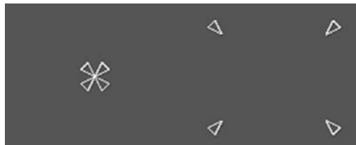
Figure 29-3. The four anchor handles for a UI element, all positioned together on the left, and the same four handles with some space between them on the right
