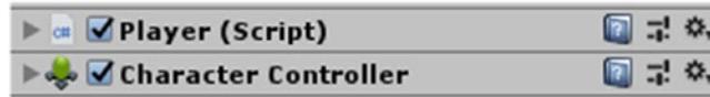
Figure 15-3. Folded Player script component and CharacterController component in the Inspector. The checkbox to the left of the component name can be unchecked to disable the component
