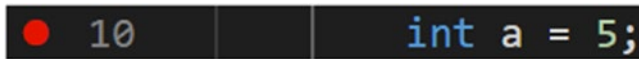
Figure 12-5. A breakpoint is added to the line of code, symbolized by the red circle at its left side
