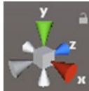
Figure 4-4. Gizmo in the top-right corner of the Scene window. The axis that the arrow corresponds to is written beside it, and each arrow is color-coded by axis
