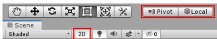
Figure 29-2. The Scene tab with the 2D button toggled on, the Tool Handle Position set to Pivot, and the Tool Handle Rotation set to Local
