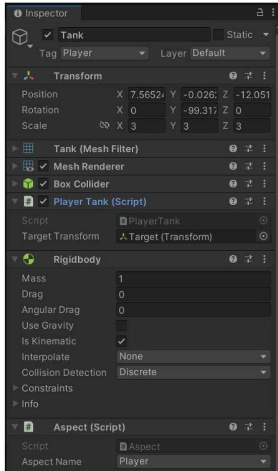
Figure 4.3 – The properties of our Tank object
