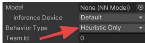
Figure 11.6 – The Behavior Type configuration
