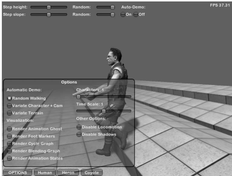
Figure 1.20 – Unity extension for inverse kinematics
