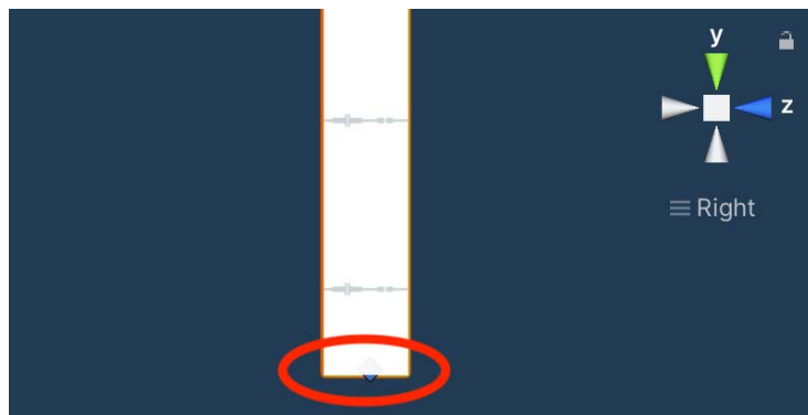
Fig. 10.10 – Center the bottom of the child prism shape at the origin. The icon can be your guide
