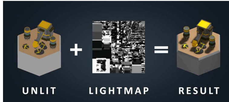
Figure 12.38: Left, a scene with no lighting; middle, a lightmap holding precalculated data from that scene; and right, the lightmap being applied to the scene
