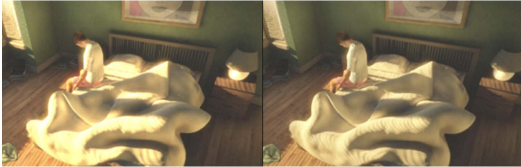
Figure 13.12: An LDR-rendered scene (left) and an HDR scene with corrected overbrights using tonemapping (right)
