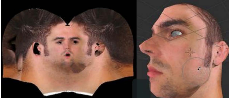
Figure 10.25: On the left, a face Texture; on the right, the same texture applied to a face mesh
