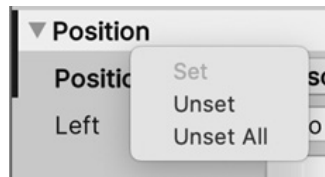
Figure 12.27 – Position is in bold, meaning it has changed. Left isn't, meaning it has the default value
