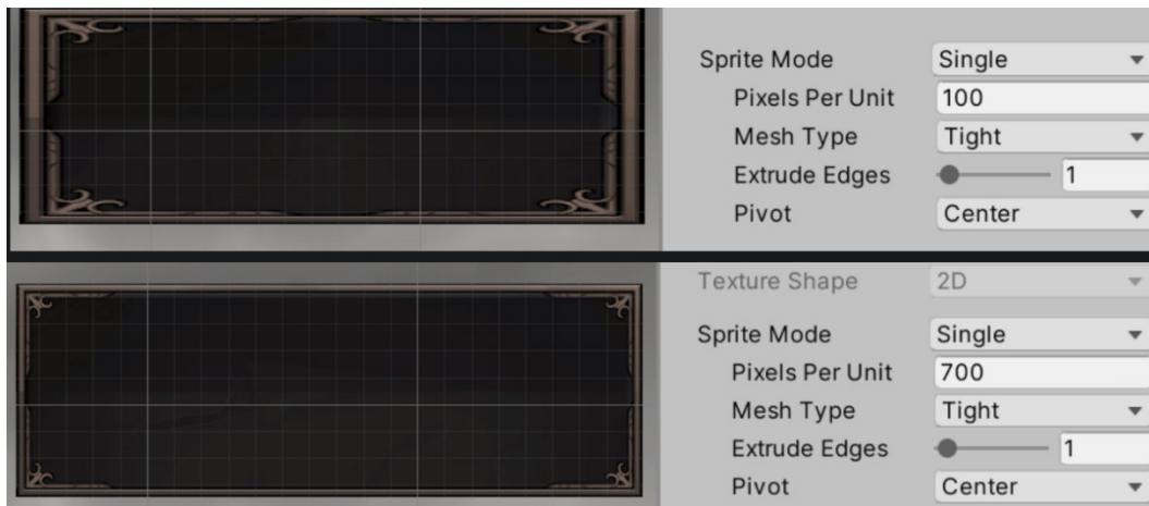
Figure 11.35 – On top, a large nine-slices image in a small RectTransform component, small enough to shrink the corners; on the bottom, the same image with Pixels Per Unit set to 700
