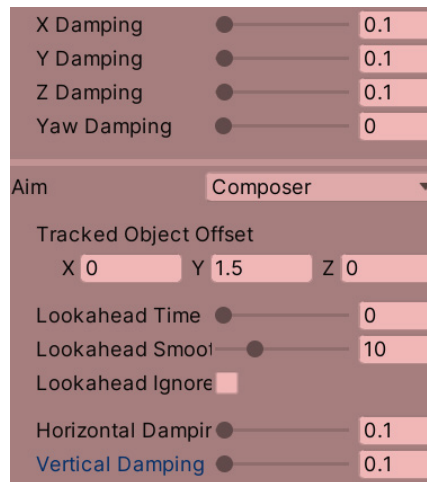
Figure 15.21 – Reduced damping of the body and aim sections of the character virtual camera
