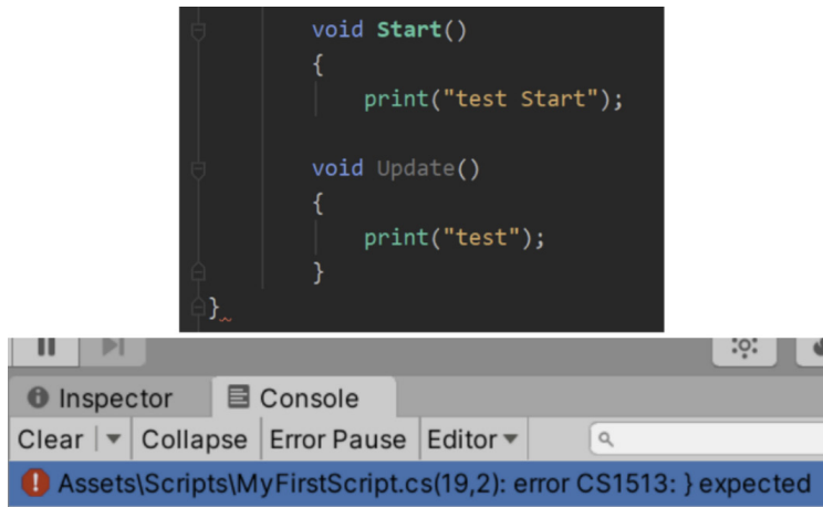
Figure 14.40 – Missing closed brackets
