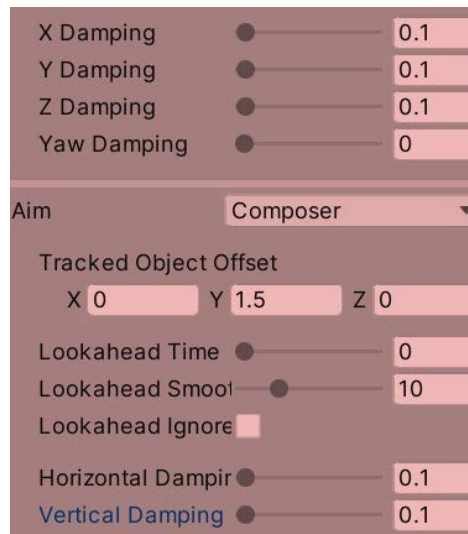
Figure 14.15 – Reduced damping of body and aim sections of the character virtual camera
