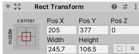
Figure 11.9 – The Rect Transform properties
