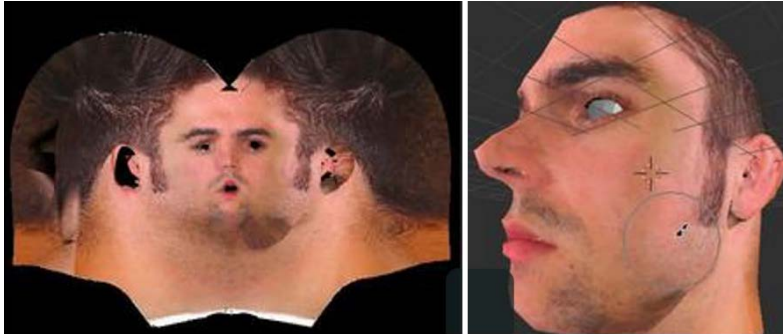
Figure 6.24 On the left, a face texture; on the right, the same texture applied to a face mesh
