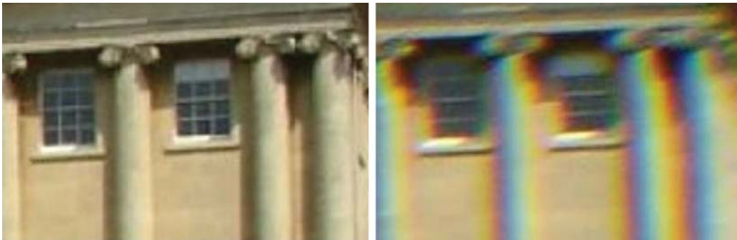
Figure 9.6 – Image without chromatic aberration (left) and the same image with chromatic aberration (right)
