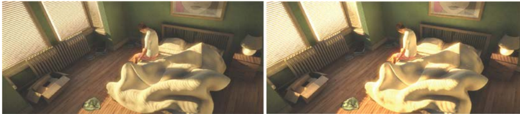
Figure 9.12 – An LDR-rendered scene (left) and an HDR scene with corrected overbrights using tonemapping (right)
