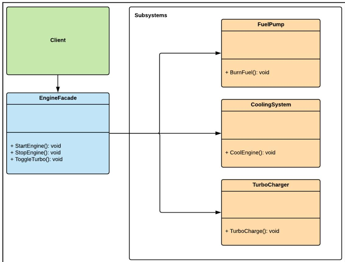
Figure 15.1 – Unified Modeling Language (UML) diagram of the Facade pattern
