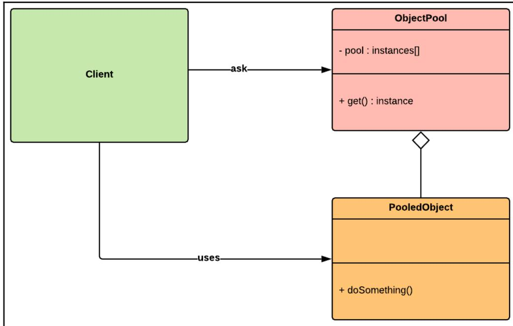
Figure 8.1 – Unified Modeling Language (UML) diagram of the Object Pool pattern
