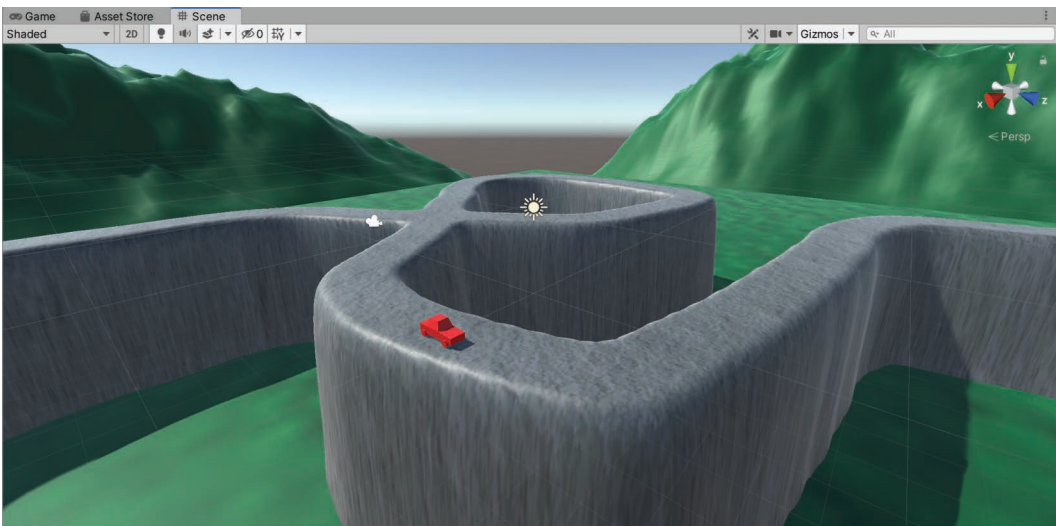
FIGURE 2.29 Normals calculated in Unity resulting in better lighting and smoother track mesh.
