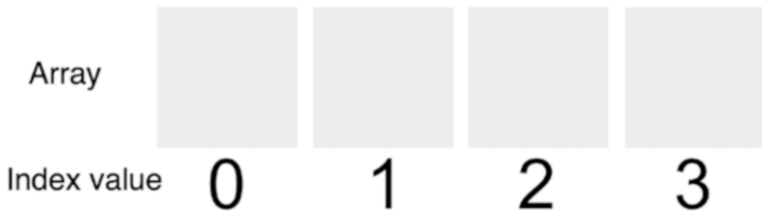
Figure 8-4. An array stores data in specific positions identified by an index number
