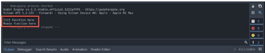
Figure 3-5. All print commands display text in the Output pane when a project runs
