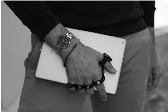
FIGURE 6.1 The TapStrap2 provides a way for a user's gestures to replicate mouse and keyboard input. ( Image Credit: TapWithUs.com. )
